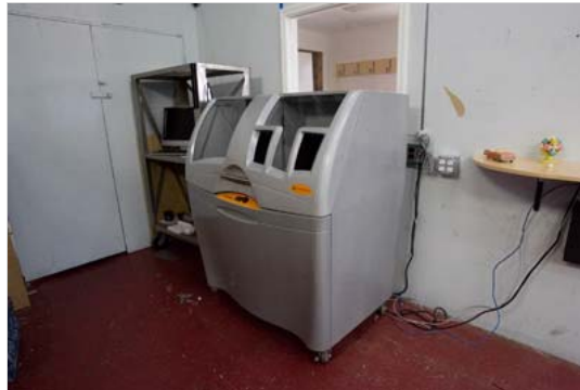
Copyright Discovery Communications, LLC The ZPrinter 450 can build a 3D model of your prototype in just a matter of hours.
