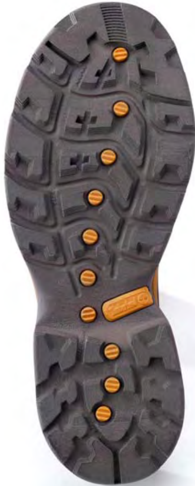
The Z Corp. Spectrum Z510 produces multicolored, highly detailed prototypes such as this Timberland sole.
